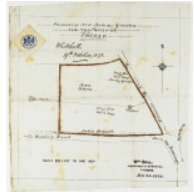
Burial boards were obliged to send a technical drawing of their proposed site, indicating where holes had been drilled to test drainage and soil composition
